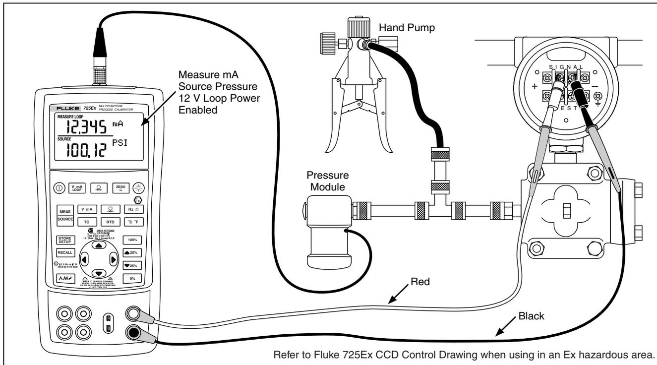
Figure 20. Calibrating a Pressure-to-Current (P/I) Transmitter
