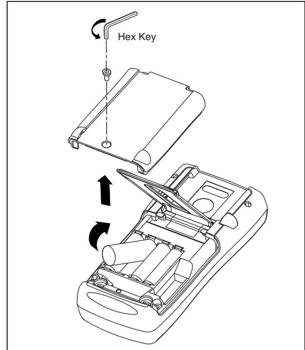
Figure 23. Replacing the Batteries
