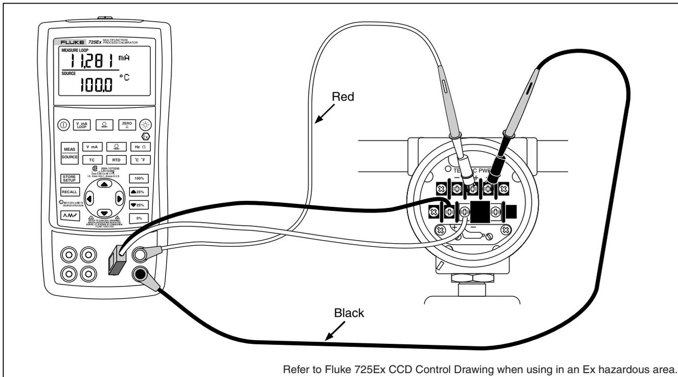
Figure 19. Calibrating a Thermocouple Transmitter
