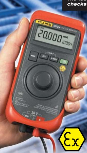
The 707Ex is an intrinsically safe loop calibrator for use in explosion endangered areas. The Fluke 707Ex is certified in accordance with the ATEX directive (Ex II 2 G Eex ia IIC T4) in Zones 1 and 2. The 707Ex is also certified to operate in accordance with Factory Mutual N.I. Class 1, Division 2 areas Group A-D.
