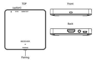
Note: the IR IN function is optional to difference Transmitter BOX.
