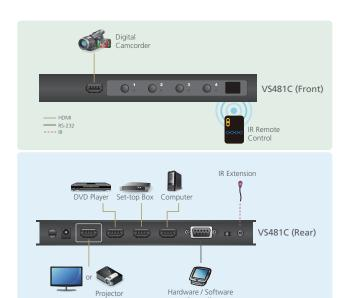
Note: Three HDMI In Ports are located on the rear panel, and one on the front.
