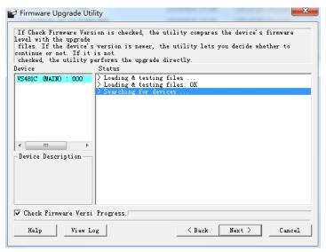
4. Click **Next** to perform the upgrade. The Port LEDs 1, 3, and 4 will flash while the upgrade is in process.
