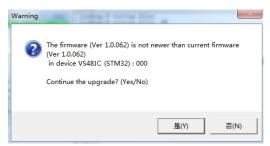
If you didn't enable *Check Firmware Version*, the Utility installs the upgrade files without checking whether they are a higher level, or not.
