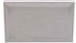
**Wall-mounted speaker** with a white wooden cabinet (RAL 9010) and metal grille. Fitted with a high-quality full range driver. Removable rear panel for easy fitting to the wall using two screws. Good music reproduction and clear speech reproduction properties. Connection to 100 volt network and level trimming by means of spring terminal. Volume control and 24 V priority relays optional.
