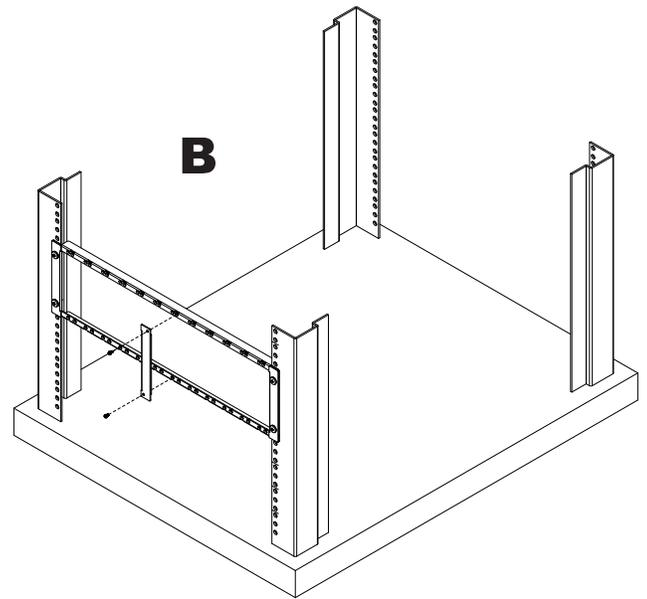
2. Place the Video Extender over the 3U Mounting Plate and bring the two pieces together so that the mounting post enters the rear hole. Next, slide the Video Extender forward to lock it in place. For video extenders without brackets, see step 4.
