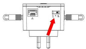
If you are using the extender in a small or medium sized space, you may not need the full power of the wireless radio. Try it, and determine if you still have sufficient Wi-Fi coverage using green mode. If so, you can save some energy.
