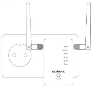
**3.** The **green** power LED will **flash** while the extender is starting up. The device is ready when the **green** power LED displays **on**.
