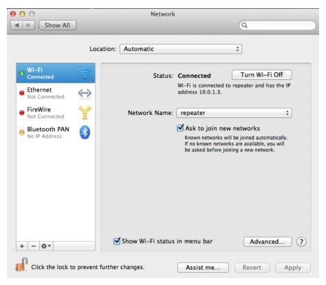
The access point should now be fully operational. The "Wi-Fi" status should display "Connected". Verify your connection by opening a web browser in an appropriate location.
