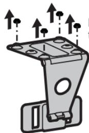
NOTE: Please remove rubber feet when mounting the stand on the wall or under a cabinet.
