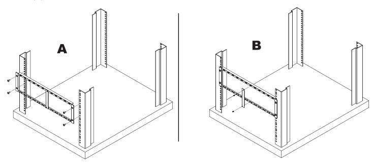
2. Place the Video Extender over the 3U Mounting Plate and bring the two pieces together so that the mounting post enters the rear hole. Next, slide the Video Extender forward to lock it in place. For video extenders without brackets, see step 4.
