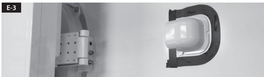
Arrange cable holder in front of (30cm apart from) antenna center by facing open side of cable holder toward projected part of the mounting plate. Then attach friction tape outside of cable holder
