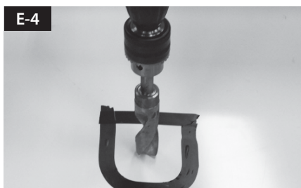
Make 15mm drill hole in the center of the tape marking
