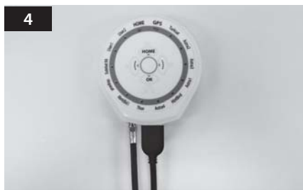
Use Power Input Cable and 5c Power Cable to Connect to Controller
