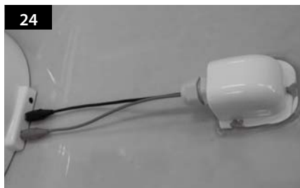
Connect black cable to the controller(middle) and grey cable to the receiver(Left).
