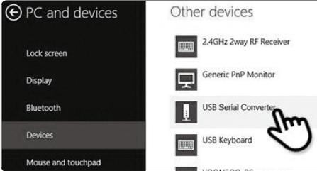
01. Connect the USB cable and turn on the controller. Please check [USB Serial Converter] port has been activated on [PC and devices].
