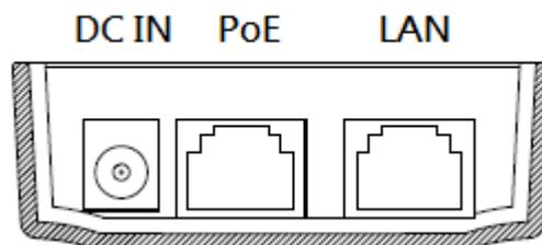
2. Use an Ethernet cable to connect the access point's LAN port to your network: router, access point or switch. If it's more convenient for initial setup, you can connect a computer directly to the access point's LAN port instead.
