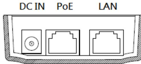
3. Connect the PoE injector to a power source using the included power adapter. Wait a moment for the access point to start up. The access point is ready when the LED is **blue**.
