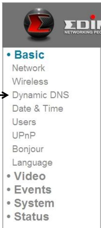
If your Internet service provider didn't issue a fixed IP address, you can use this function to report your current IP address to a dynamic DNS service provider, so you can locate your network camera without having a fixed IP address.
