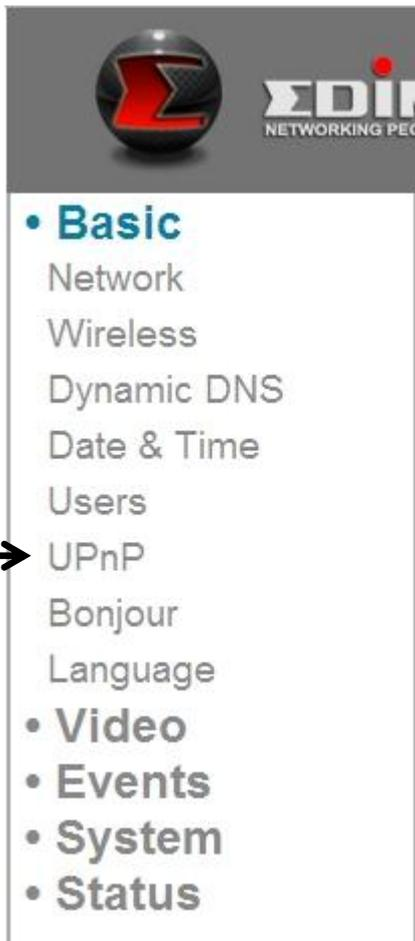
When you enable this feature, Windows computers can discover this network camera from Windows Network Neighbor directly, and you don't have to know this network camera's IP address in advance (This only works on the local area network).
