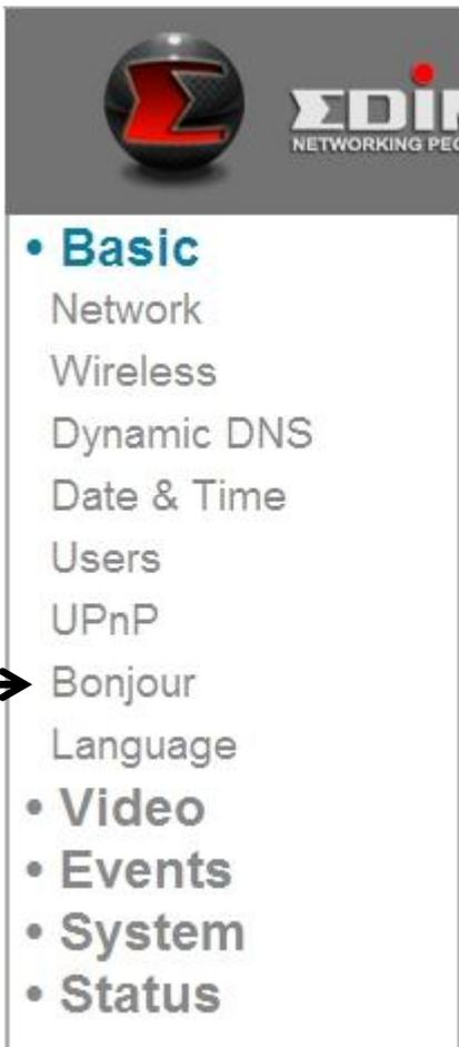
When you enable this feature, Macintosh computers can discover this network camera from the Safari web browser directly, and you don't have to know this network camera's IP address in advance (This only works on local area networks).
