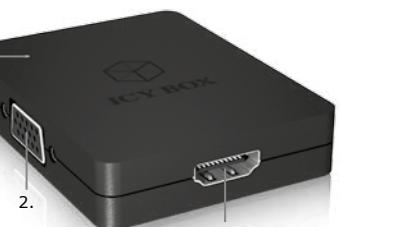
**1. LED Indicator** to indicate linking status with monitor
