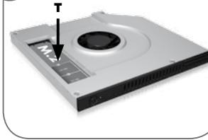
Attach the M.2 card with provided screws.
