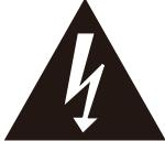
A triangle with a lightning symbol draws the user's attention to "dangerous voltage" without insulation in the cabinet which may be high enough to entail a risk of electric shock.
