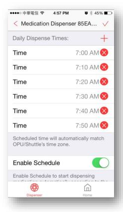
3. When programming is complete, tap "✓" in the upper-right corner. The system will ask the user to press the "Sync" button on the medication dispenser. Before tapping "OK", press the "Sync" button on the medication dispenser. After pressing the "Sync" button, LED 2 should turn red for a second.
