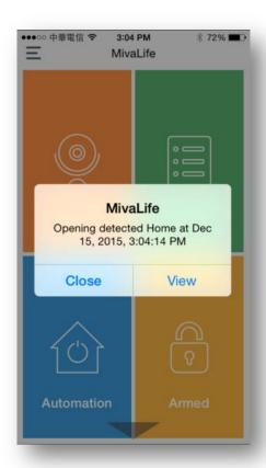
In Armed status, when the garage door has been opened and the sensor detects that the pitch has been tilted more than 45°, an in-App mobile alert will be sent to you immediately.
