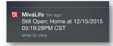
A "Still Open" notification will be sent if the garage door has been left opened for a while, no matter whether the system is Armed, in Stay Mode, or Disarmed.
