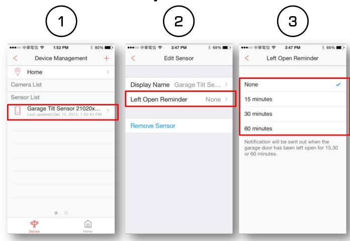
In Device Management, select the "Garage Tilt Sensor" you want to edit. Tap 'Left Open Reminder'. Then set the notification interval from 15 to 60 minutes.
