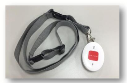
Attach the lanyard and wear the fall detector as pendant.
