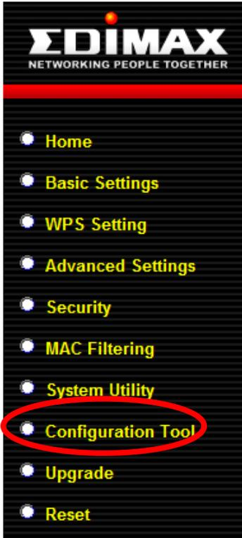
The access point’s configuration tool enables you to back up the current settings, restore the settings to a previously backed up version or reset the access point back to its original factory settings.
