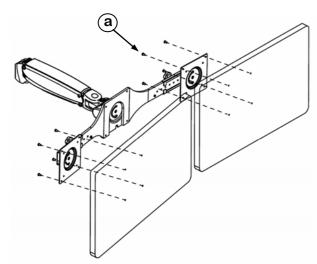
Adjust the pivots along the wings to fit your monitors. Tighten Hand Knobs to fix the Pivots.
