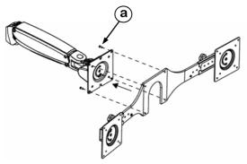
2 Attach two monitors to the Extended Pivots.
