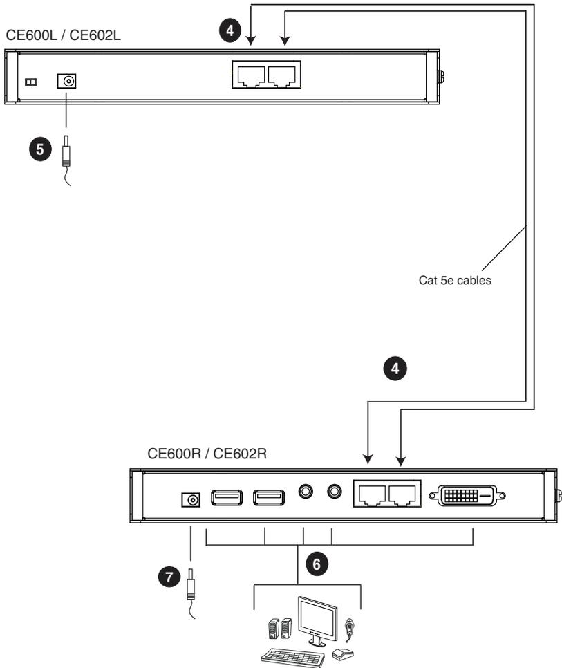
**Note:** 1. The serial port on the CE600L / CE602L connects to the computer; the serial port on the CE600R / CE602R (not shown) connects to a serial device (optional).
