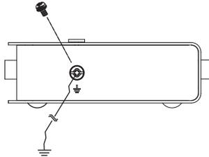
2. Make sure that the computer that the Local Unit connects to and the monitor that the Remote Unit connects to are properly grounded.
