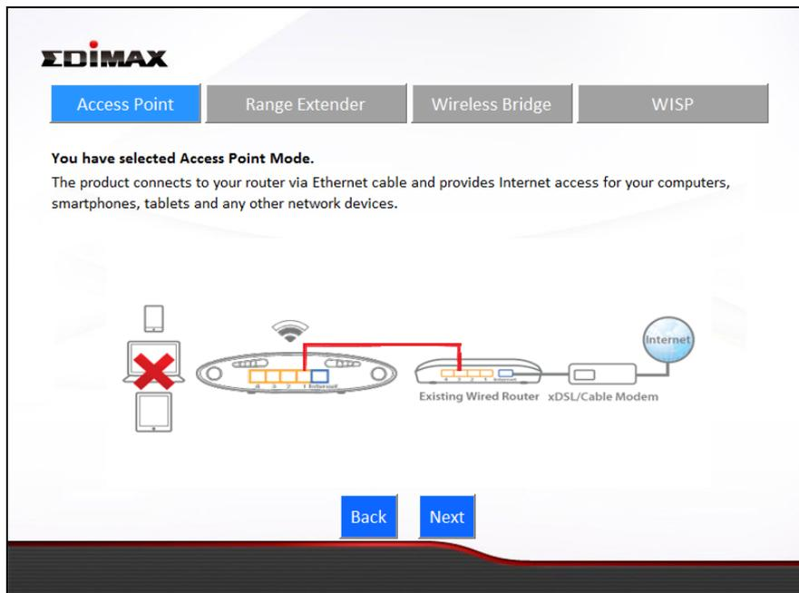
2. Connect the **yellow** LAN port of your BR-6208AC to the LAN port of your existing router using an Ethernet cable, then click “Next”.
