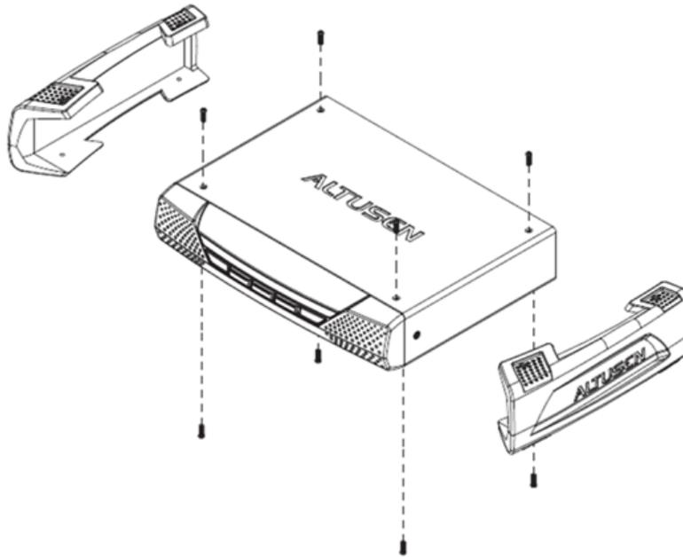
2. Remove the bottom and side screws from the KE6900.
