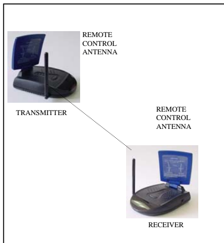
Fig-4: How to orienting the remote control antenna
