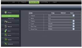
1. **Live:** Allow you modify channel name, Position, Show time and Record time. If show time is set to <disable>, current system time will not appear on the screen on Live mode; and if record time is set to <off>, system time can't be found in the record file.
