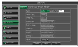
When selecting Static from the Type, user can directly input IP address, Subnet Mask, Gateway and DNS shown as below picture 5-32.
