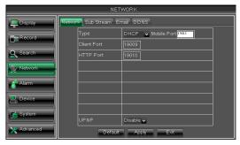
When selecting DHCP from the Type, A router will automatically allocate IP address for your DVR. After restarting each time, the IP address captured by your DVR may be different. So, port forwarding is required when you visit a remote DVR.
