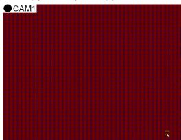
The channel will be separated into a 44x36 grids (PAL/NTSC mode). When any object moves into the motion detection area, and the area where the object is located is displayed in red and motion detection will be triggered. In the semi-transparent area the motion detection is not activated.
