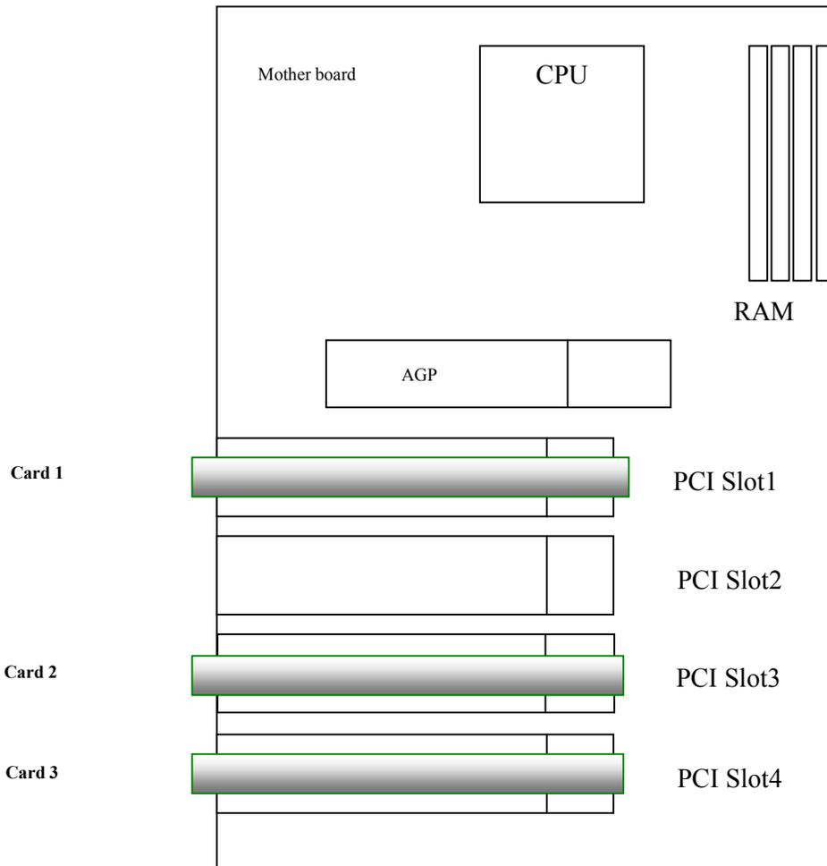
**Note:** When installing multiple cards in a single PC the total video channels may not exceed 24 cameras. The proper card order is shown as below. The card nearest to CPU will be the first card. Only card 1 need to be connected for Watch Dog connection (see following page).
