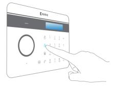
Input user code or admin code first, then press the [Disarm ①] button, the system enters disarm state when one beep is heard and the disarm LED Indicator lights on.
