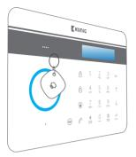
The control panel has a RFID reader for unlocking the electronic door lock by disarming the system. Just place the RFID tag close to the RFID reader, the green LED indicator flashes once.
