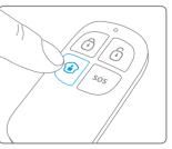
Press [Stay • ] button on the remote control, the system enters home mode when one beep is heard and the home mode LED is on. All the normal sensors are armed except the home mode sensors which are disarmed, so that users can move freely at home.
