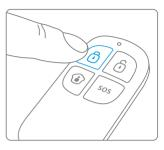
Press the [Arm ① ] button, the system enters arm state when one beep is heard and the arm LED on the control panel is on.
