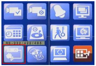
Press (on DVR remote controller) to set the <u>Baud Rate to be 2400</u>. (That's the key point to let standalone DVR & Speed Dome communicate each other.)
