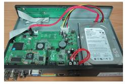
3. Hold the SATA HDD, and use a screwdriver to fix it as shown
