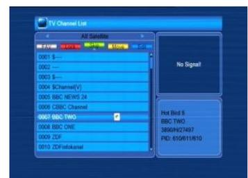
6. Press the yellow key to move the move the button upward. Select the programme and press the OK key to mark this programme with the move marker. Press the PR+, PR- keys to move the cursor to the position where you want it and press the OK key to confirm. Press the yellow key again to exit from yellow mode, and you will find the yellow button returned to its original position.
