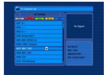
5. Press the green key to move the skip button upward. Select the programme and press the OK key to mark this programme with the skip marker. You can cancel this marker by pressing the OK key once more.
