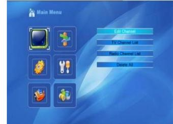
During the installation the OK key confirms a selection and the LIST key shows a Drop Down Box if the column has a ◀▶ mark. You can also use the numeric keys on the remote control (RCU) to enter a numeric value.
