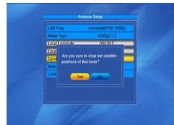
4. Motor Settings: Press the OK key to enter the Motor Settings window. Satellite: Press the  $\leftarrow$   $\rightarrow$  keys to select the circled satellite. Or press the OK key to open the drop-down list, then select the desired satellite in the list and press the OK key to confirm. Transponder: The same operation as above.
