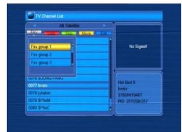
4. Press the red key to move the lock button upward. Select the programme and press the OK key to mark this programme with the locked marker. You can cancel this marker by pressing the OK key once more.
