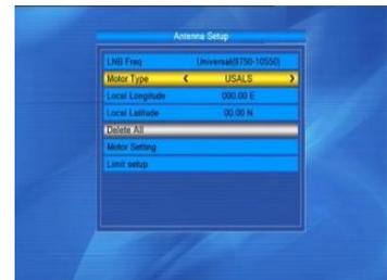
7. Motor settings: Press the OK key to enter into the Motor setting window.
