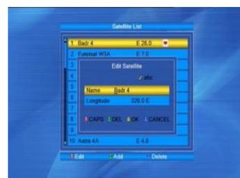
Longitude: You can press the  $\triangleright$   $\triangleleft$  keys to switch between east longitude and west longitude. After pressing the OK key, you can use the numeric keys to edit the longitude, press the EXIT key or the PR+, PR- keys to exit editing mode. The range of the longitude is from 1 to 180 degrees. If beyond this range, the system will inform you "out of range" when you press the yellow key on the RCU.
