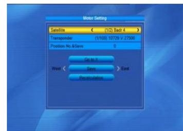
Position No., & Save: The range is from 0 to 63. “0” denotes the original position. You can select the proper value when you rotate the antenna.
