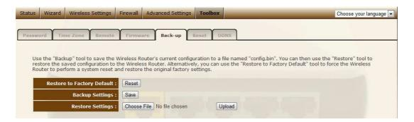
Use the "Backup" tool to save the Broadband router current configuration to a file named "**config.bin**" on your PC. You can then use the "Restore" tool to restore the saved configuration to the Broadband router. Alternatively, you can use the "Restore to Factory Defaults" tool to force the Broadband router to perform a power reset and restore the original factory settings.
