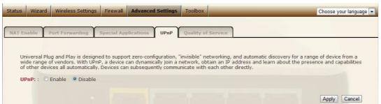
**UPnP Feature** You can enable or Disable the UPnP feature here. After you enable the UPnP feature, all client systems that support UPnP, like Windows XP, can discover this router automatically and access the Internet through this router without having to configure anything. The NAT Traversal function provided by UPnP can let applications that support UPnP connect to the internet without having to configure the virtual server sections.
