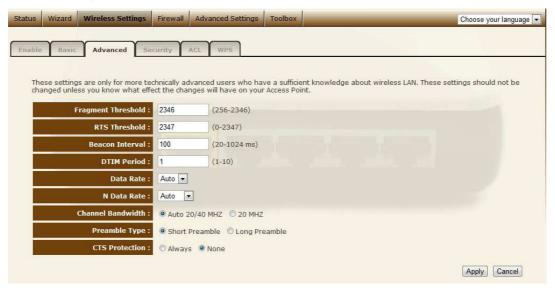
**Fragment Threshold** "Fragment Threshold" specifies the maximum size of a packet during the fragmentation of data to be transmitted. If you set this value too low, it will result in bad performance.
