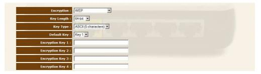
**Key Length** You can select the WEP key length for encryption, 64-bit or 128-bit. The larger the key will be the higher level of security is used, but the throughput will be lower.
