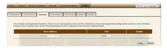
**Host Address** This is the IP address of the host in the Internet that will have management/configuration access to the Broadband router from a remote site. If the Host Address is left 0.0.0.0 this means anyone can access the router's web-based configuration from a remote location, providing they know the password.
