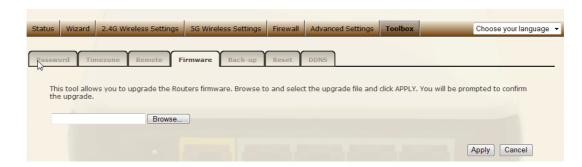
**Firmware Upgrade** This tool allows you to upgrade the Broadband router's system firmware. To upgrade the firmware of your Broadband router, you need to download the firmware file to your local hard disk, and enter that file name and path in the appropriate field on this page. You can also use the Browse button to find the firmware file on your PC.
