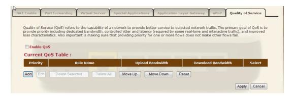
**Enable/Disable QoS** You can check "Enable QoS" to enable QoS functionality for the WAN port.
