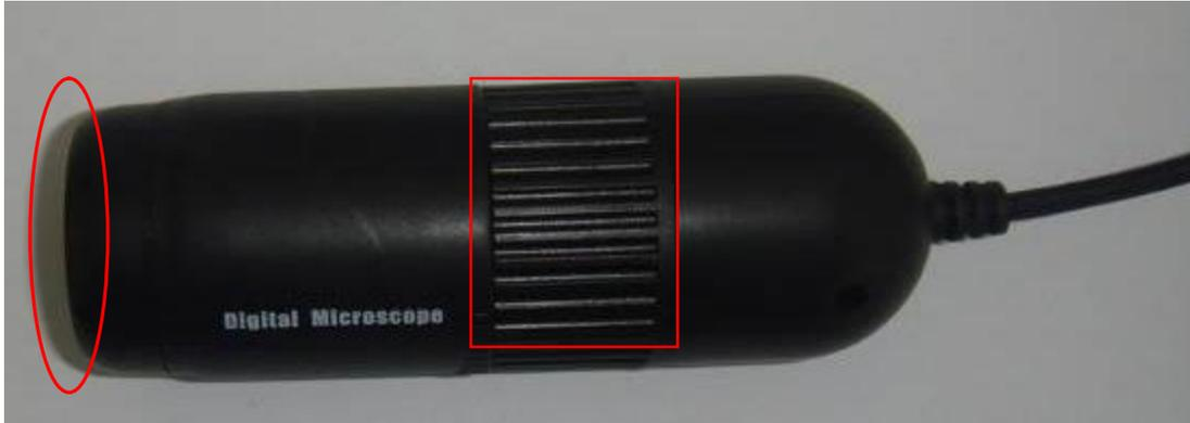
In the figure, a red box shows the focus ring of the microscope camera. The lens side of the microscope camera is shown in a red oval line. This end should be closer to the object for getting a large magnification view.
