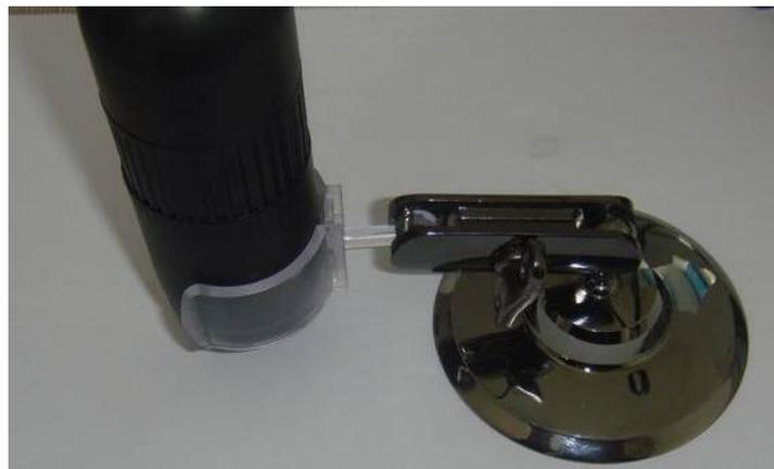
**Placement when not using the microscope**
