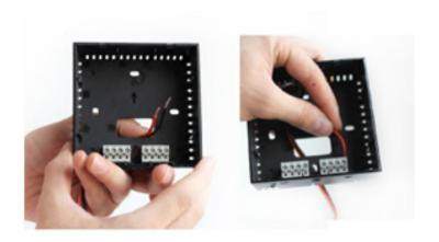
6 With the help of a screwdriver put the wires in proper position, considering the marks will be inside the casing.
