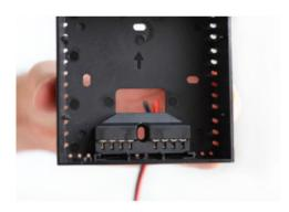
7 Close the Smart Thermostat momit housing. Take the front of momit Smart Thermostat. You will see at the top there are protrusions that, together with the back part of the housing, will work as a hinge. Place it properly and support the rest of the thermostat by pressing gently. Press until the tabs at the bottom of the housing make a clicking sound, as sign that it has been wedged properly.
