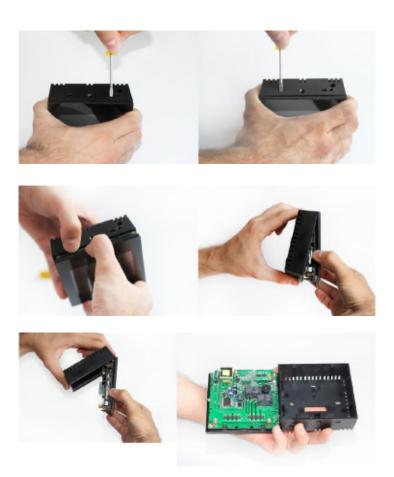
Remove the back of the housing. There will be labeled positions where the cables of your heating and/or air conditioning must go. You will also see several openings in which will be the fixings of the thermostat to the wall.
