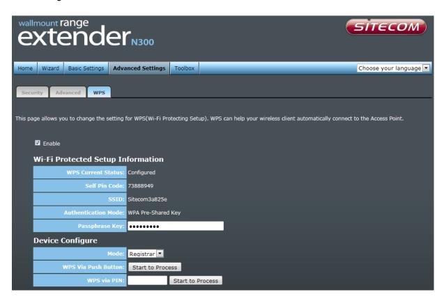
Check the box to enable the WPS function and uncheck it to disable the WPS function.
