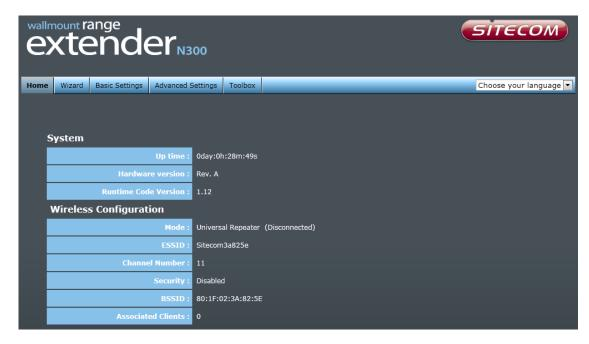
The System status section allows you to monitor the current status of your device, the UP time, hardware information, serial number as well as firmware version information is displayed here.
