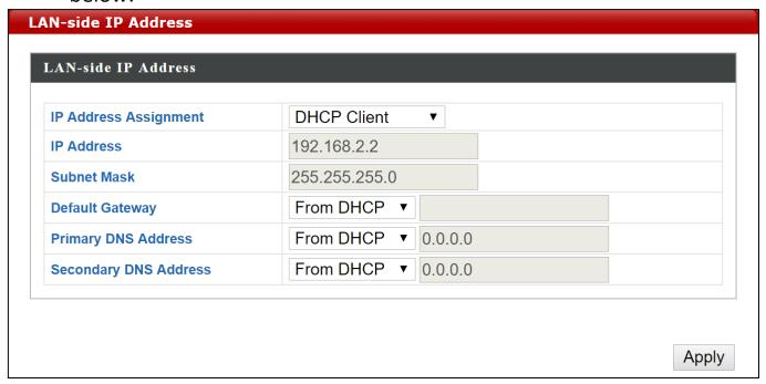
2. Enter the IP address settings you wish to use for your access point. You can use a dynamic (DHCP) or static IP address, depending on your network environment. Click "Apply" to save the changes and wait a few moments for the access point to reload.
