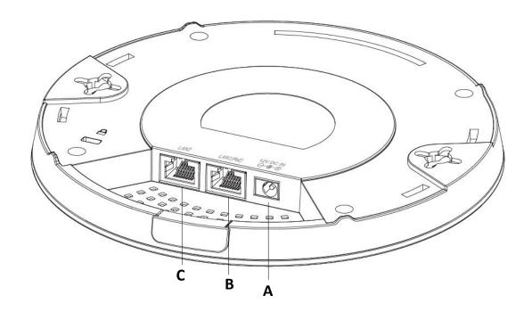
A 12V DC IN 12V DC port to connect the power adapter
