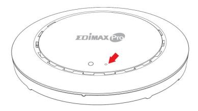
**2.** Wait for the access point to restart. The access point is ready for setup when the LED is **blue**.
