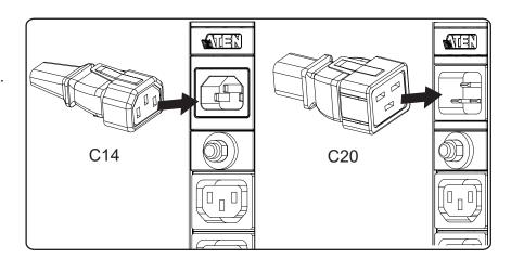
3. To disconnect the plug from the PDU, grip the plug and squeeze the EZ-Lok tab as you pull the cord from the outlet.
